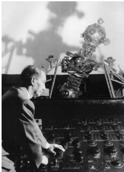
The Zeiss projector used 1,000 watt lamp to project the stars. Today, it's displayed at Carnegie Science Center.
